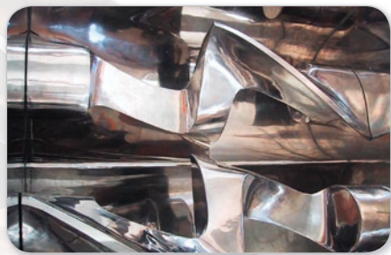
Double Sigma arms made in Stainless Steel and polished.
