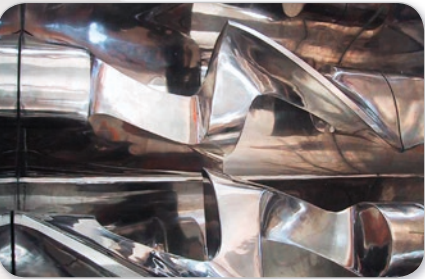
Double Sigma arms made in Stainless Steel and polished.
