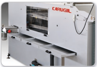
Hygienic desing. Scraps are collected onto three easily removable trays.
