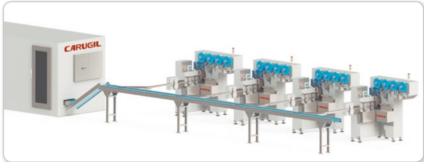
Several wrapping machines can be combined with one tunnel through synchronization trays.
